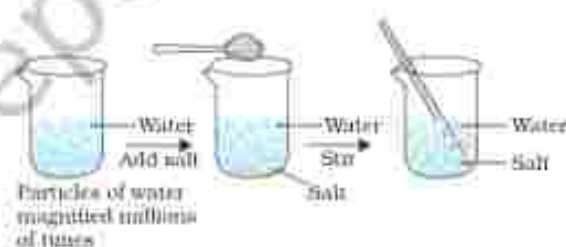
Fig. 1.1: When we dissolve salt in water, the particles of salt get into the spaces between particles of water.
